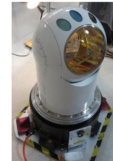
23cm / 28kW Helicopter Beam Director Subsystem
