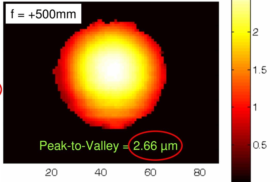
The measured wavefront amplitude matched within 2%
