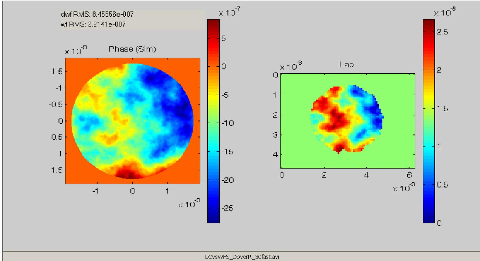
***The measurements from the Shack-Hartmann wavefront sensor that were processed by WaveTrain matched the phase screen written to the LC within the noise floor of the sensor.***
