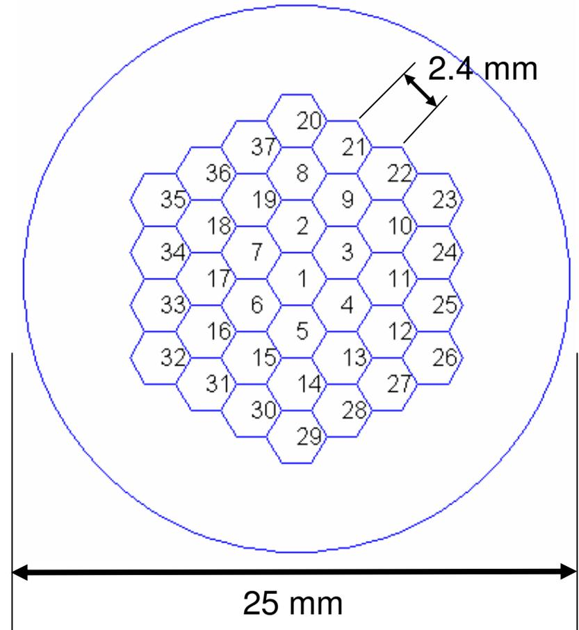
**NOTE: Assumed actuator size = 80% of actuator separation**
