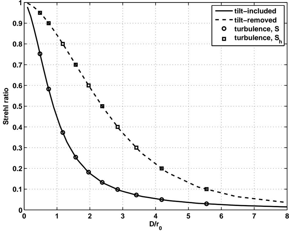
Figure 1: Tilt-included Strehl ratio ( $S$ ) and tilt-removed Strehl ratio ( $S_h$ ) with  $D/r_0$ .
