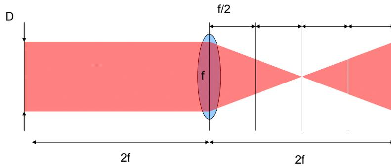
**Figure 4 - Example 4-f Imaging System**
