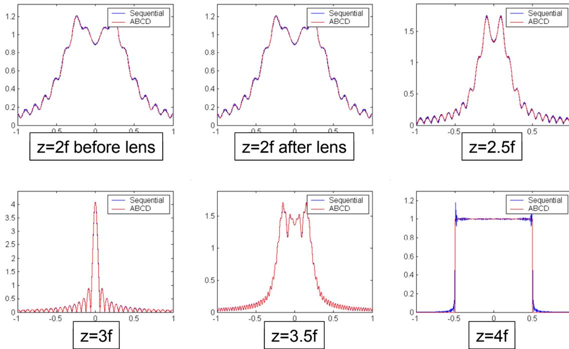
**Figure 5 - Field amplitudes for the modeled planes of the 4-f imaging system**
