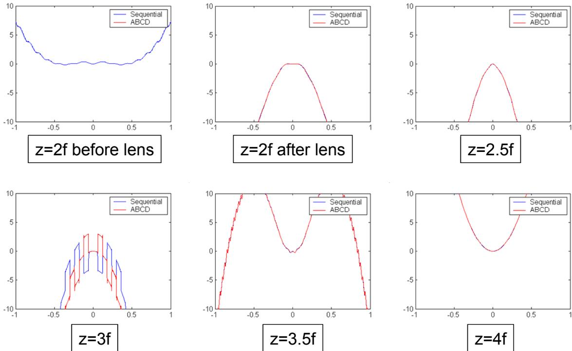
Figure 6 - Unwrapped 1D phase profiles (in radians) of the target planes of the 4-f imaging system
