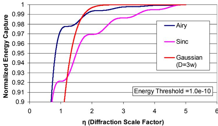
Figure 2 - Energy capture comparison of diffraction scaling factors
