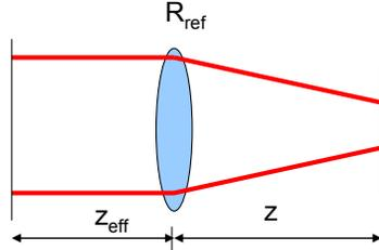
**Figure 1 - Effective optical diagram for spherical wave propagation**
