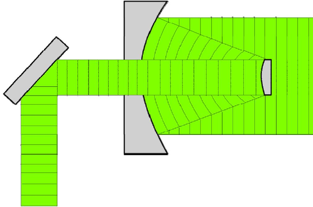
To first order, ordinary lenses and mirrors operate only on the overall tilt and/or curvature of wavefronts passing through the optical system.
