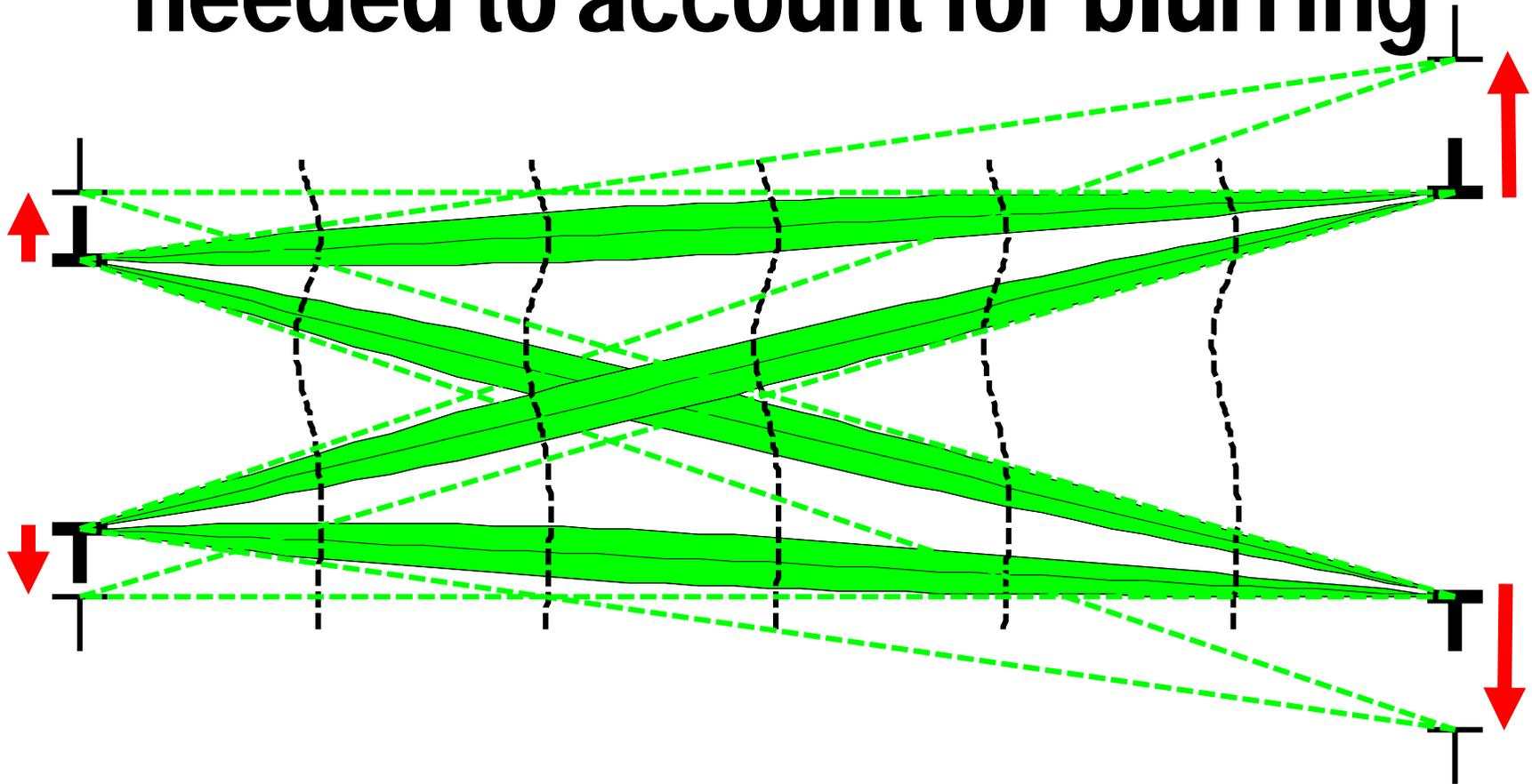
Blurring effects due to diffraction or propagation through aberrating media have the effect of enlarging the apparent size of the source aperture, as seen from the receiver, and vice versa.
