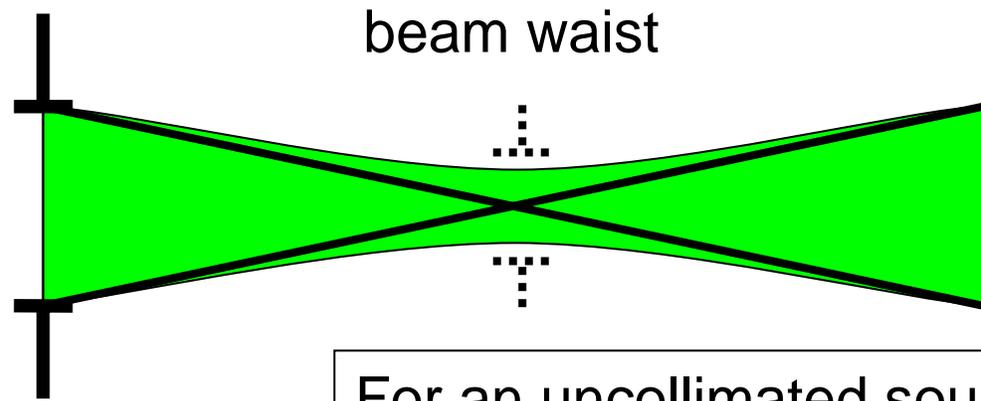
For an uncollimated source, the receiver entrance pupil provides a second limiting aperture, and the receiver FOV may provide a third, at the image plane.
