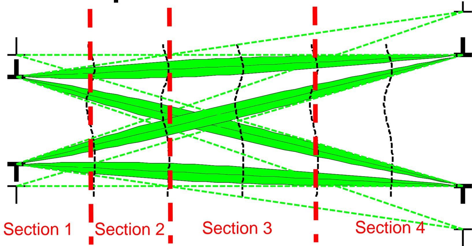
Blurring effects vary with position, changing the sizes of the blurred apertures. For example, at the source the set of rays to be modeled is limited by the unblurred source aperture and the blurred receiver aperture, while at the receiver it is limited by the unblurred receiver aperture and the blurred source aperture.
