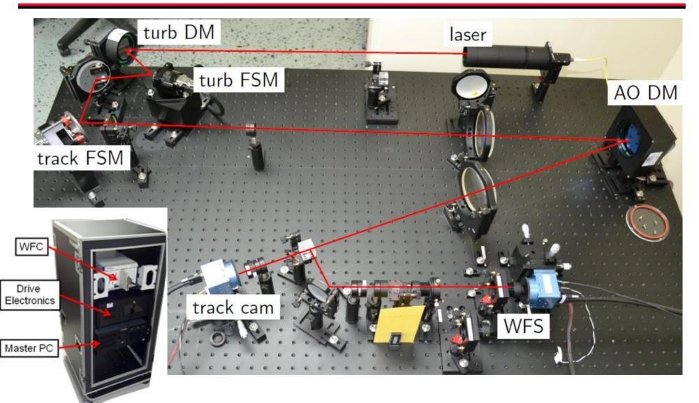
Full system including deformable mirror, high-speed wavefront processor, and track+AO controls built by MZA
